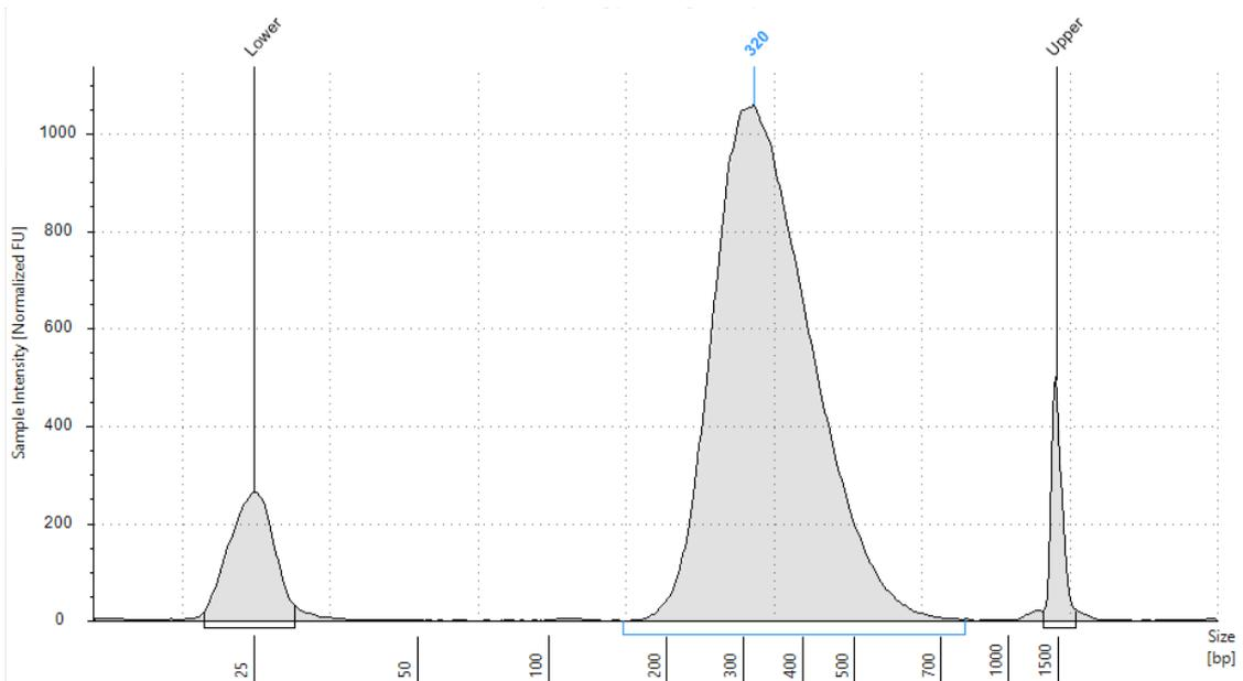
**Figure 4:** Analysis of amplified capture DNA pool using an Agilent High Sensitivity D1000 ScreenTape assay. The electropherogram shows a maximum peak in the size range of approximately 310 – 330 bp (+/- 20 bp).
