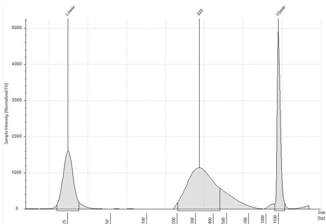
**Figure 2: Analysis of amplified prepared library DNA using an Agilent D1000 ScreenTape assay. The electropherogram shows a maximum peak in the size range of 310 - 330 bp (+/- 20 bp).**
